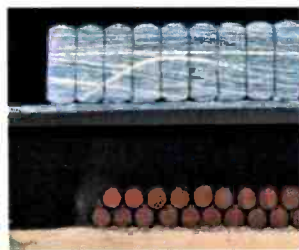
The voice coil consists of flat aluminum conductor wire wound on-edge on an aluminum core, eliminating the inefficient air gaps between the round copper windings of a conventional voice coil.
