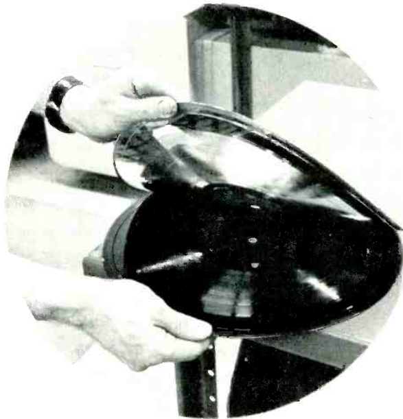
The silver mother is carefully stripped from the master lacquer.
