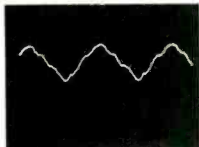
A—Shows output of low frequency driver when driven at a freq. of 22 Hz. Sound pressure reading, 90 dB. Note poor wave form.
