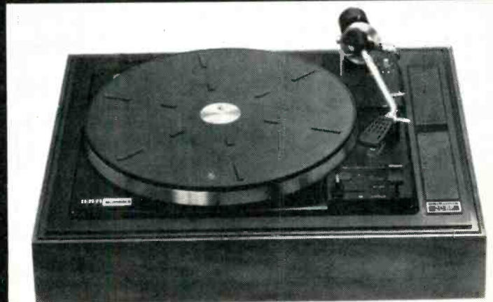
BSR 20 BPX—Automated single-play belt-drive turntable
