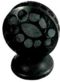
Fig. 11 —Western Electric 1B housing.
