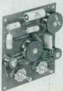
Close-up View of 3/way Integrated Crossover Network
