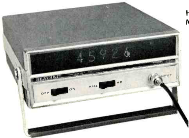
Fig. 1—Note the simplicity of the controls—only two rocker switches, one for power and the other for switching from Hz to KHz.
