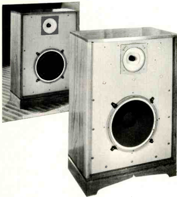
Fig. 2—The completed system, with a mirror showing the back side, which is identical to the front.
