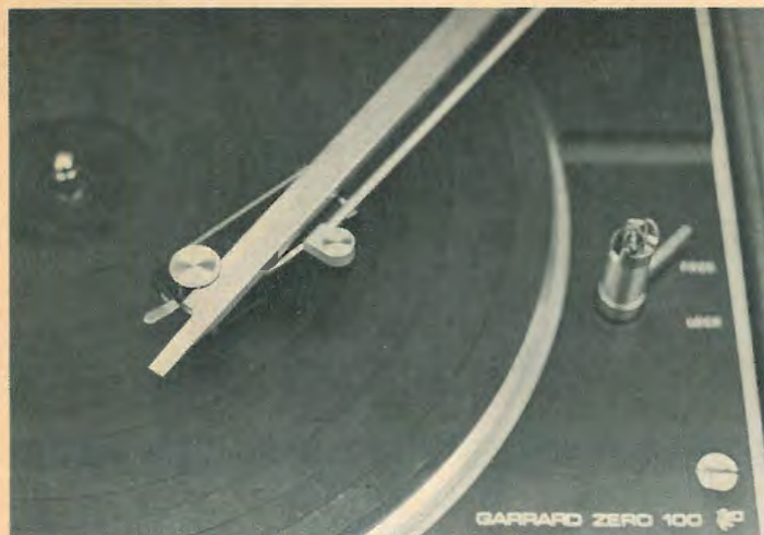
Fig. 1—When the arm is near the center grooves of the record, the angle is changed by the controlling tubular component at the right. This part is pivoted on the rear of the head and provides practically perfect tangency throughout the entire record.
