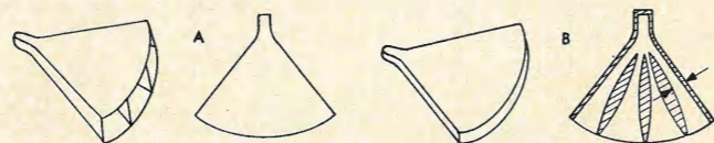
Fig. 12—A, sectoral horn; B, diffraction horn.
