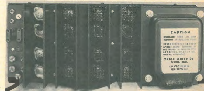
Fig. 1—Rear view of the amplifier with one protective perforated metal shield removed from one group of transistors. All input and output connections are made at the left end of the unit.
