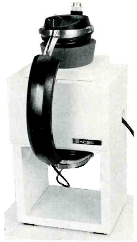
Fig. 1—Koss artificial ear. Dark portion is molded rubber and provides the requisite 6 cm 3 cavity.
