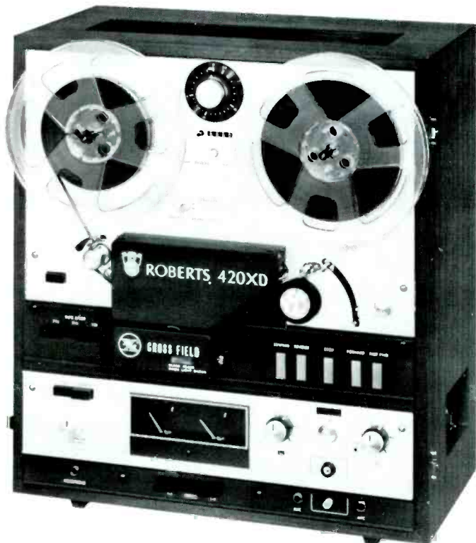
Fig. 1—Roberts Model 420XD Tape Recorder—a deck with auto reverse, four speeds, and a host of other features in one machine.
