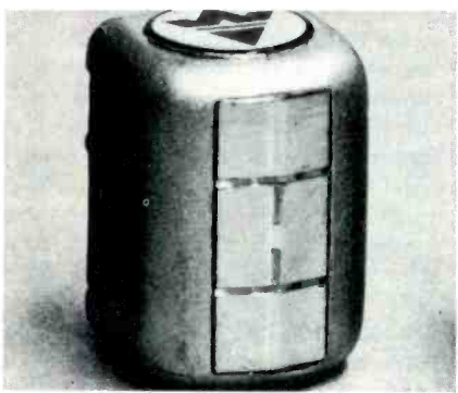
Fig. 3—A stereo head in close-up shows the gap formation. Note the head contouring and the grooves near tape edge location of the stereo head. These grooves act as a suction device when tape is moving past, but can trap oxide if not kept scrupulously clean.
