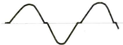
Fig. 2—Primary crossover distortion.
