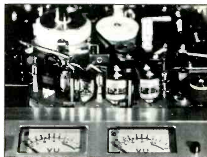
Fig. 2. The recorder with the top plate and head cover removed.
