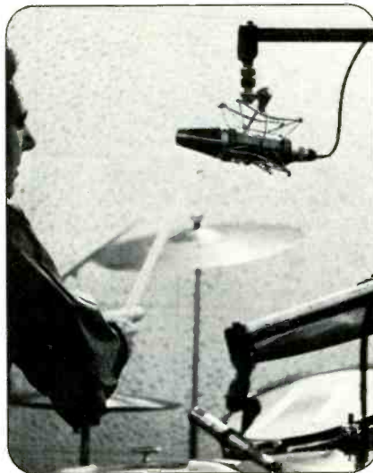
Fig. 3—Al Rogers on drums. A Neumann model 67 is used here over the cymbals, with a Neumann model 56 to capture snare-drum sounds.
