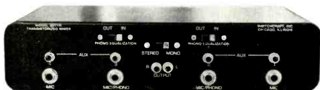
Fig. 6—Front and rear views of Switchcraft model 307TR transistorized mixer.
