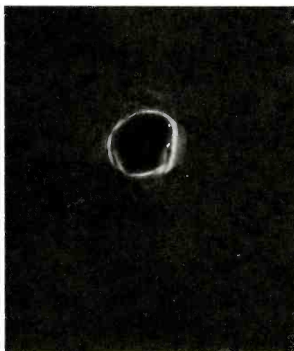
Fig. 12—Spherical tip after life test without skating-force compensation.
