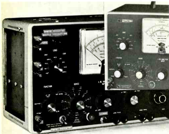
Fig. 3—Modified audio analyzer compared to original, “mono” audio analyzer. Note additional outputs and switches.
