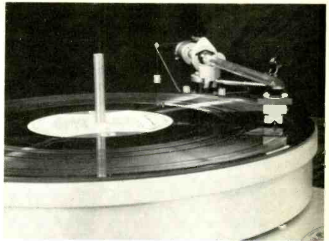
Figs. 4 and 5—Skating-force detector in Shure SME tone arm illustrates how it operates without bias compensation or anti-skating force (left) and with satisfactory bias compensation (right).
