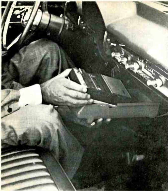
Fig. 4. The optional "Car-Mount" accessory which provides r.f. output to feed any AM car radio on an unused frequency.
