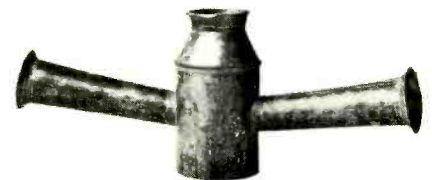
Fig. 7. "Triple" mouthpiece used by Bell in conjunction with a magneto telephone to transmit vocal music over telegraph wires between Paris and Brantford, Ontario, during the summer of 1876.
