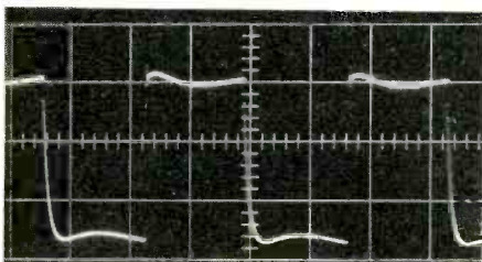
Fig. 15 (A). Multivibrator output measured at the junction of 1.8k- and 200-ohm resistors. Vertical sensitivity: 0.5 volts/cm; horizontal sweep: 100 \mu sec/cm. Per cent flutter: 0.25% rms; flutter rate 90 Hz (Sweep: from left to right).
