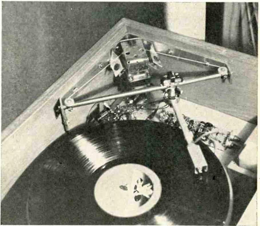
Over-all view of the servo groove tracker mounted in the corner of a turntable cabinet. An experimental preamp is seen just behind the arm, while the servo amplifier is located underneath the motor assembly.
