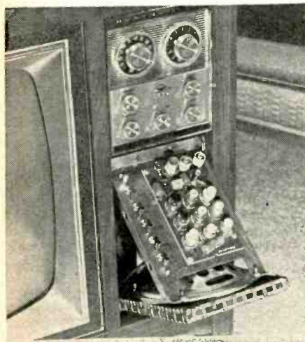
Fig. 3. Service and convergence controls are front accessible when the speaker panel is tilted forward
