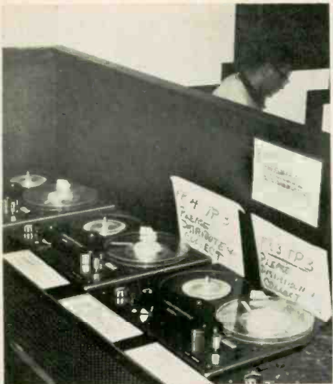
(Left), Bank of three Tandberg tape recorders employed as the master program source and (Right), Master console at The George Washington University showing the instructor's control panel at the left and the thirty-two individual student control strips.
