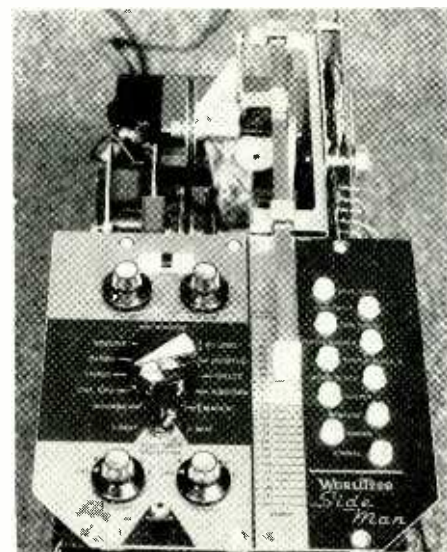
Fig. 6. Control panel and tempo level bar of Side-Man.
