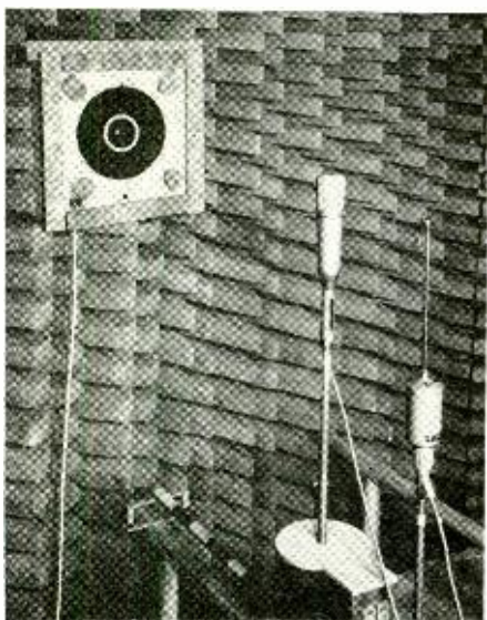
Neumann measuring set-up, with MM 5u calibration microphone in foreground and U 67 in measuring position on turntable (nearest loudspeaker) in anechoic chamber
