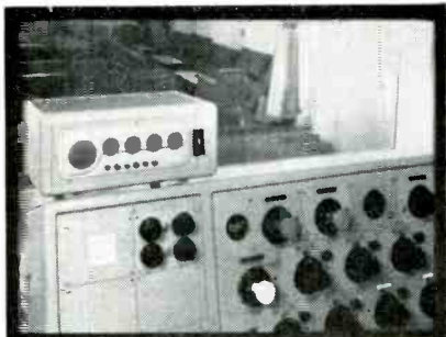
A studio control room where the programmes are passed through a QUAD control unit for special balancing.
