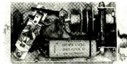
Fig. 2. Very low voltage relay assembly. Note heat sink on rectifier.
