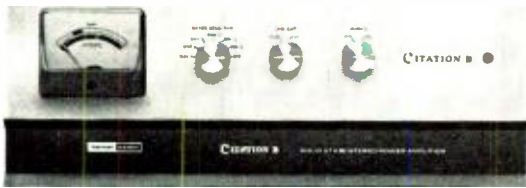
Handsome front panel; facilitates custom installation. Features include current-adjustment meter, on/off switch with pilot light and low-cut filter. Removable bottom panel conceals idling adjustment controls.
