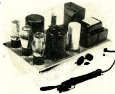
Fig. 1 Regulated power supply built by author. Unit provides heavily filtered and regulated voltage to bias oscillator and recording amplifier of tape recorder.
