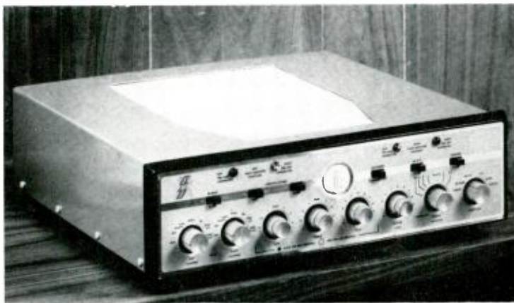
Fig. 5. E.M.I. Stereoscope amplifier. The name comes from the use of a small cathode ray tube as an output indicator.
