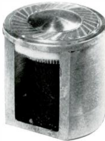
Fig. 2. The complete omnidirectional microphone unit without its housing.
