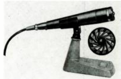
Fig. 13. The cardioid microphone with its housing and holder.
