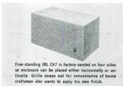
Custom-installation version of JBL C47 has snap-on grille that overlaps enclosure 1/2" on all four sides to cover gap between enclosure and wall framing or cabinet opening.
