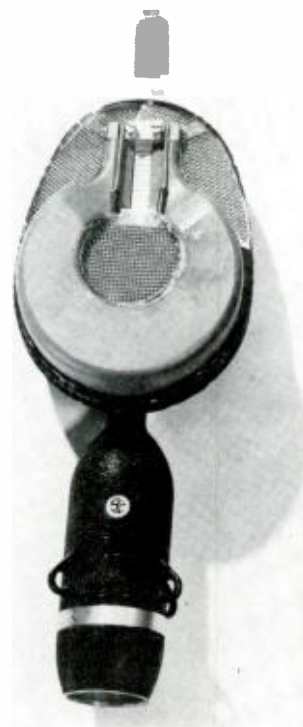
Fig. 6. A high-quality ribbon microphone with the outer case and the inner ribbon damping gauzes removed.
