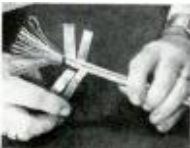
Shielding cables reduces magnetic radiation or pickup.
