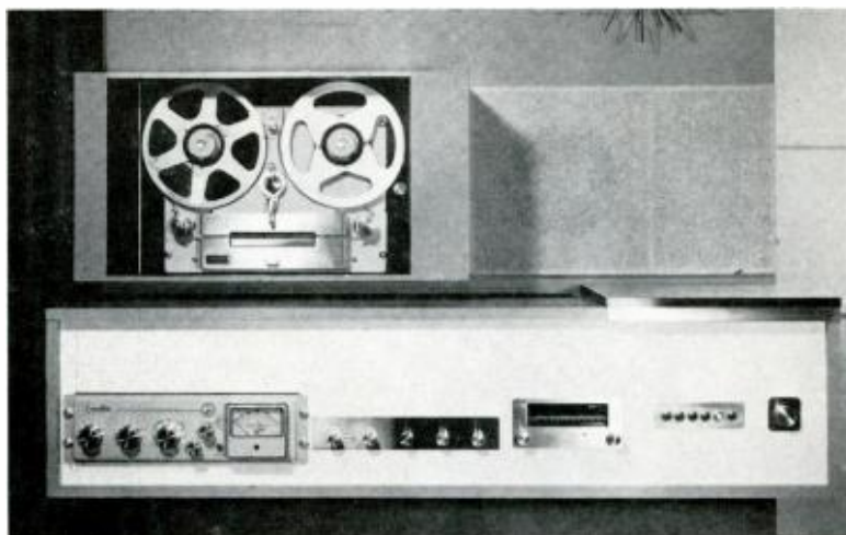
Fig. 2. Aluminum “Flexdoor” provides access to tape recorder, actuates light switch in completely open position.
