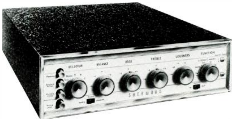
Fig. 1. Sherwood Model S-4400 stereo preamp with a single 36-watt power amplifier.
