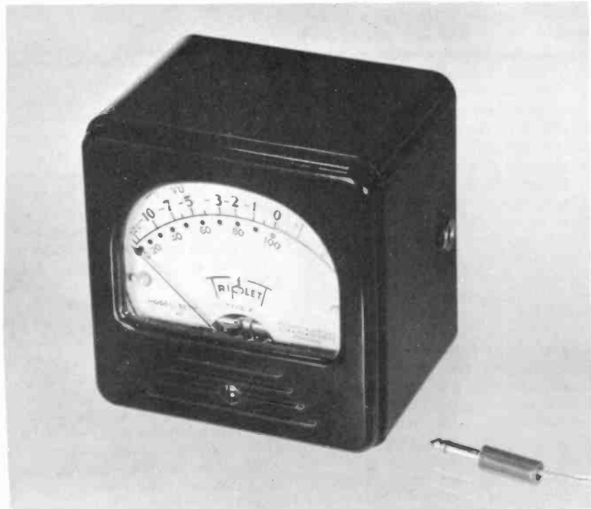
Fig. 1. A typical modern VU meter. Most meter manufacturers make one or more models of VU meters.
