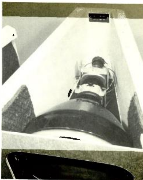
Fig. 13. Mounting of picture tube in compartment, showing relative position of various components.
