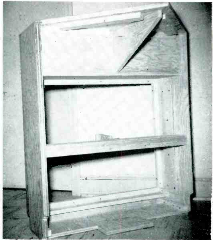
Fig. 4. Another view of the frame. Having no back, it must be firmly attached to the walls.
