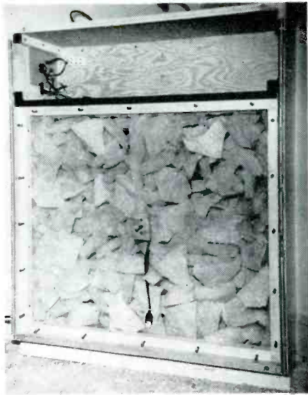
Fig. 6. Before attaching the loudspeaker mounting board, the entire interior is filled with pieces of fiber glass.
