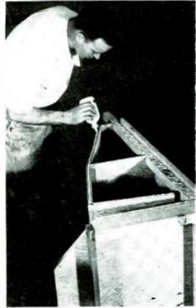
Fig. 9. In addition to the liberal use of casein glue, as shown here, it is desirable to caulk all joints with a non-hardening compound, such as linoleum cement.
