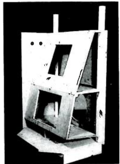
Fig. 7. The structure progresses—part C, with the large rectangular speaker-access opening, has been installed. Note space between lower shelf and corner posts.
