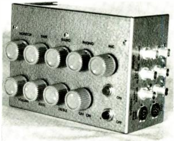
Fig. 7. Battery-powered control unit has phono preamplifier, four channel mixer, and tone controls.
