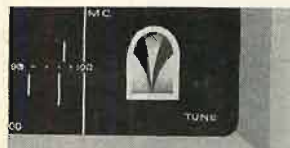
Precision-ray tuning eye makes it simple to tune precisely on both AM and FM.
