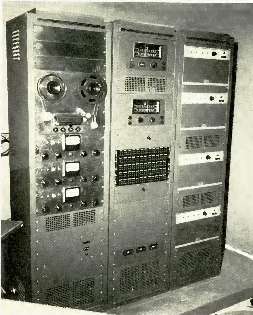
Fig. 4. The control room is provided with Rek-O-Kut turntable, three-channel Ampex recording and playback mechanism, two Altec FM-AM tuners, and four power amplifiers in addition to complete control console.
