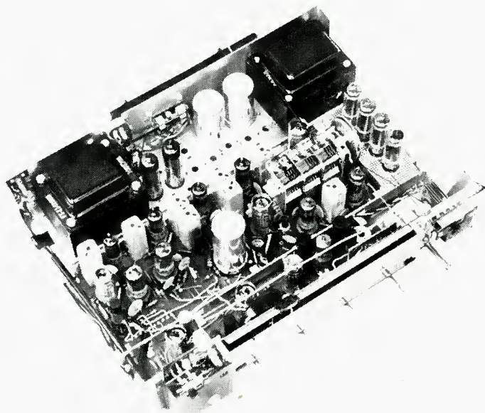
Fig. 1. Harman-Kardon receiver chassis constructed with the printed-wiring techniques described. Performance is held to extremely close limits.
