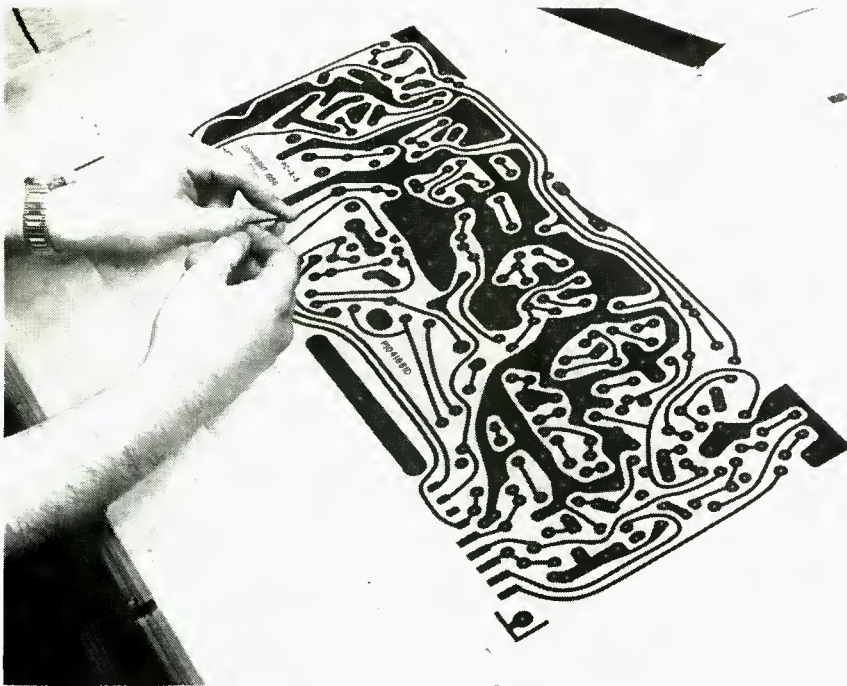
Fig. 2. Method of making mock-up drawing which serves as master for production of printed-wiring panel. Pressure sensitive tape is used for laying out "wires" between connection points.
