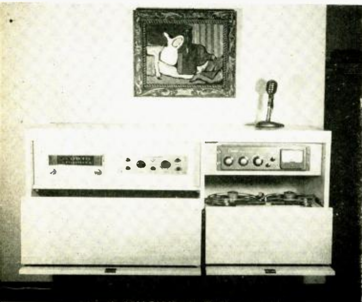
Fig. 2. The system controls are free of mechanical crowding, control knob bunching or cute disguising. They are mounted in flush furniture-finished panels, easily removable by loosening a few countersunk brass wood screws.
