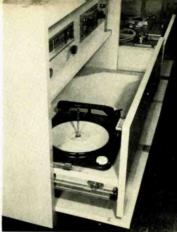
Fig. 6. No Tin Pan Alley is this vista of audio instrumentation, but rather a Rue de la Hi-Fi. Space alongside automatic record player is provided for addition of heavy-duty turntable in future. Control panel is recessed for knobs to clear doors when closed. Note spring catch in near edge of door.
