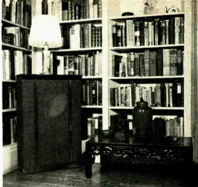
Fig. 3. Heard with "presence" but not seen is the 12-inch duplex Stentorian speaker with 11½ pound magnet. Plenty of excursion for clean lows through Cabinart's KR-4 Klipsh-designed folded horn, and tweeter to highs with separate coaxial-mounted voice coil. (The camera "saw" the speaker, but we are not a camera!)
