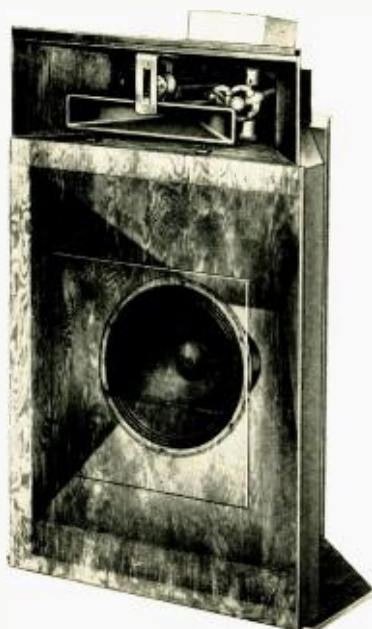
Fig. 8. Phantom view of low-frequency section topped by the diffraction horn and its three sections—each of which covers a specific frequency range.
