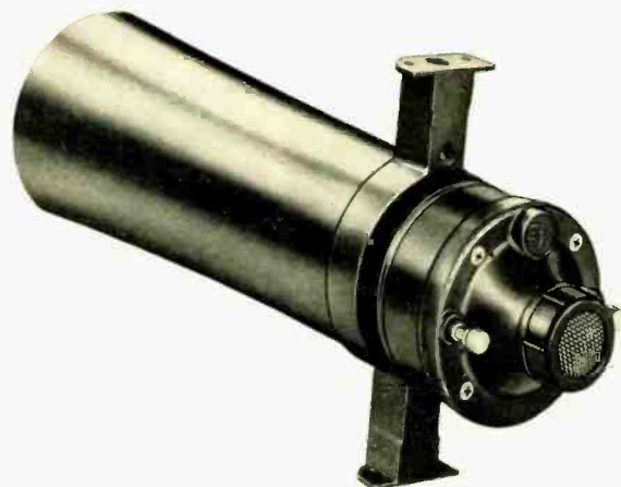
Fig. 5. One of the two mid-bass driver units assembled to its phenolic three-pass folded horn. Two of these units "exhaust" into the large diffraction horn of Fig. 3.
