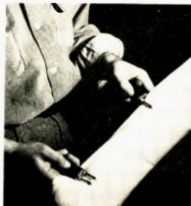
Fig. 2. Plugs can be polished on a long strip of cloth saturated with jeweler's rouge.
