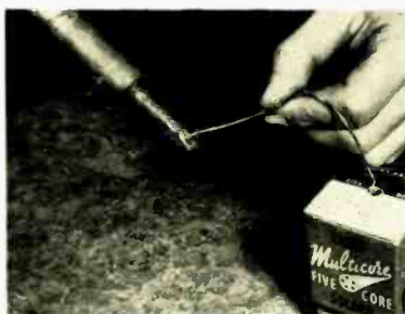
Fig. 1. A new iron or one which has lost its brightness should always be tinned. Clean the tip to brightness with sandpaper or a fine file and apply cored solder, making sure it adheres to the entire tip surface. If a tip is untinned it will not conduct heat to the work.
