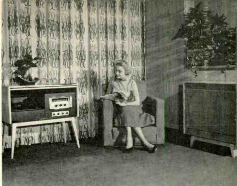
Fig. 4 (right). A compact two-unit music system. Equipment cabinet is simple in design, yet completely functional and attractive. Basic power amplifier is mounted into the speaker enclosure on the right. (Courtesy R.C.A.) Fig. 4A (above). Outline sketch of components pictured in Fig. 4.
