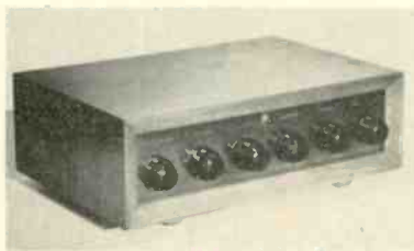
A complete preamplifier and control unit which utilizes the filter circuit described.
