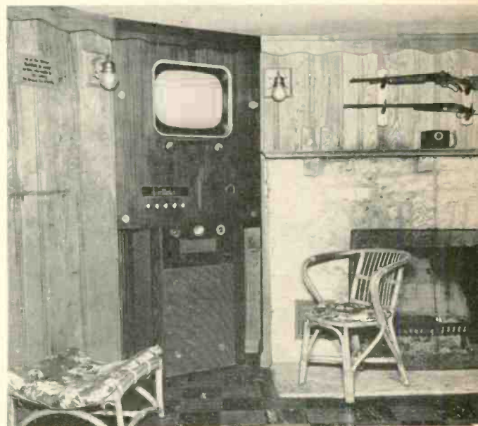
Fig. 11. Here is a simple but very effective manner of installing a complete system into a small area providing an ideal corner for a loudspeaker and a very advantageous location for the television unit. (Courtesy Radio Craftsmen.)
