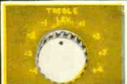
Control #2 Treble Eight indicated stages... over a 23 db range, without distortion.
