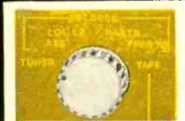
Control #1 Input selector Six positions: Tuner, Tape, AES, NARTB, FFRR, COL. LP. The latter four positions provide equalization for all records.
