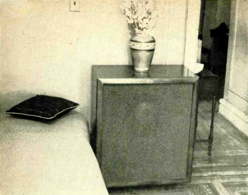
Fig. 5. The bass-reflex cabinet is placed independently and permanently in the city apartment. Contains a 15-inch coaxial speaker with crossover network at 2000 cps. HF balance control (rolloff) unit is mounted on the back panel.
