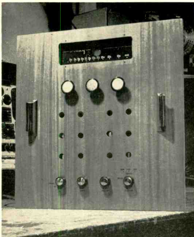
Fig. 3. Face of panel shows ventilating holes in a symmetrical pattern, balancing with the tuner control knobs above and the amplifier control knobs below. Hand grips at each side are heavy brass, serve to lift out the panel and the equipment secured on its inner face.
