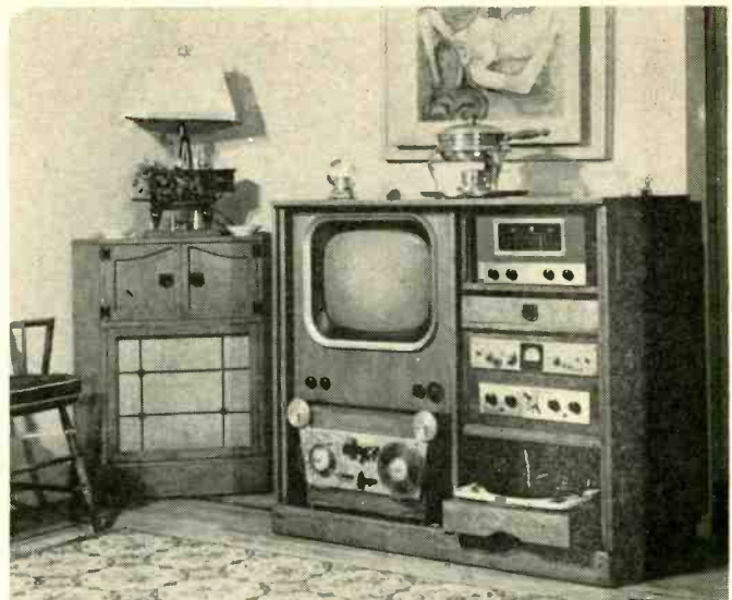
Fig. 12. A complete music system from pickup to tape recorder, with a corner bass-reflex speaker enclosure adjacent. Styled in Early American Colonial accented with Dutch influence, this unit is quite compact, measuring 48 in. wide, 42 in. high, and 24 in. deep. See chart of minimum dimensions, Table 1.
