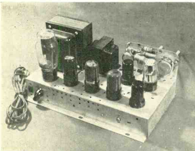
Fig. 3 (left). The entire amplifier, including preamplifier, is on a single chassis with the power supply. Fig. 4 (right). The underside view shows that the space is well utilized.
