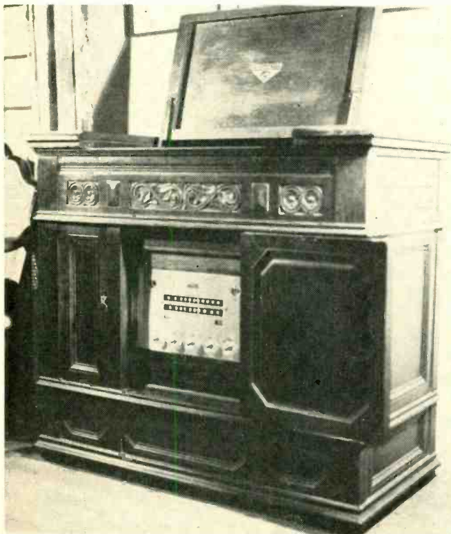
Fig. 11. An "old-timer" brought up to date. An early Electrola cabinet modified to house a radio tuner, amplifier, and transcription turntable. (Photo by the author)
