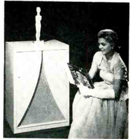
Fig. 53. This is the enclosure made by Karlson Associates of Brooklyn, N. Y. It is not a horn but derives its effect from coupling an inside air column to the outer air through a slot of an exponential shape.
