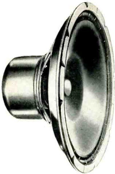
Fig. 9. One method of attacking the dual problem of high- and low-frequency reproduction with a single speaker is illustrated by this Permoflux speaker. The cone is relatively rigid for good treble but slitted at the frame for bass compliance.
