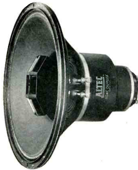
Fig. 18. The coaxial speaker is a two-way system in minimum space and often at minimum expense. This Altec 604C is the latest version of one of the first and best coaxials. It requires a crossover network just like separate dual systems.
