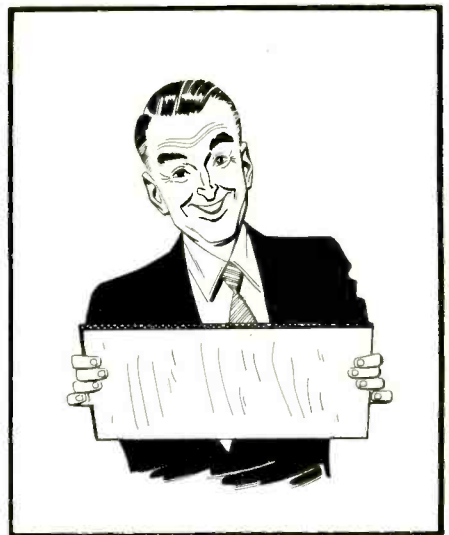
Fig. 6. A piece of cardboard held in both hands simulates a stiff cone. It remains fairly rigid when the hands move fast, acting as a piston to displace air. While good for high frequencies, its low compliance as a cone raises resonance.
