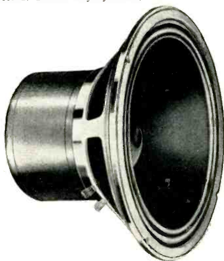
Fig. 12. This photograph shows a typical high-quality woofer—low-frequency speaker. This one is the Electro-Voice 15WK, a 15-inch cone unit with resonance at low 32 cps and a 5¼-lb. field magnet to give uniform flux over a large area.
