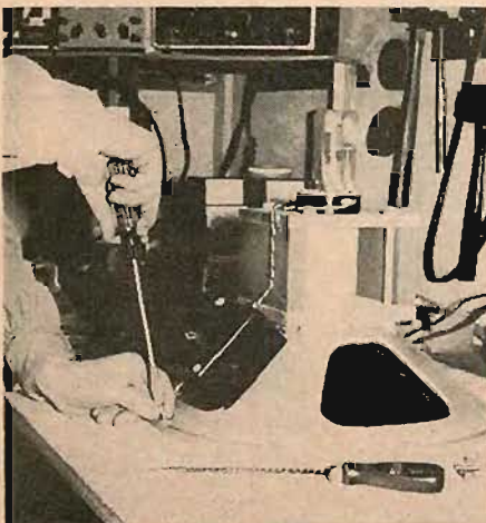
Fig. 8. Demonstration of fastening of speaker to its baffle. Note long screwdriver for ample leverage to drive screws home for absolutely firm fit. Bolts are recommended, to avoid risk of speaker frame working loose in time and vibrating against baffle when in operation.
