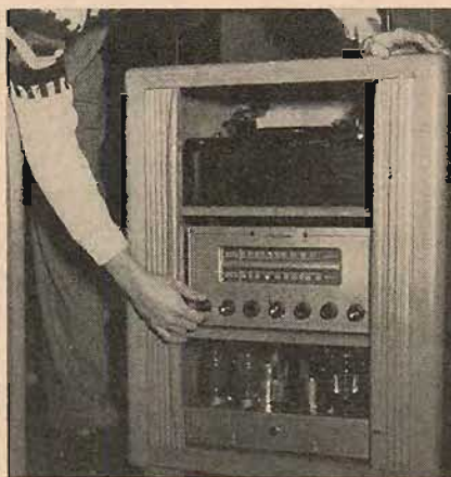
Fig. 6. Cabinet with tambour doors parted to show record changer on top shelf; tuner with controls on middle shelf; amplifier unit below it. Speaker is in separate cabinet.
