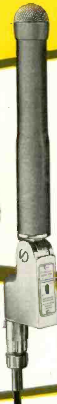
MODEL 654 DYNAMIC Response 50-13,000 cps, \pm 2.5 db. Power rating —55 db*. Omnidirectional. 50-250 ohm impedance selector. Integral breath-blast filter. List, $95 Net, $57
