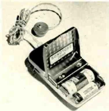
Fig. 3. Battery compartment provides space for both A- and B-batteries, and hinged door gives access to fitting controls.
