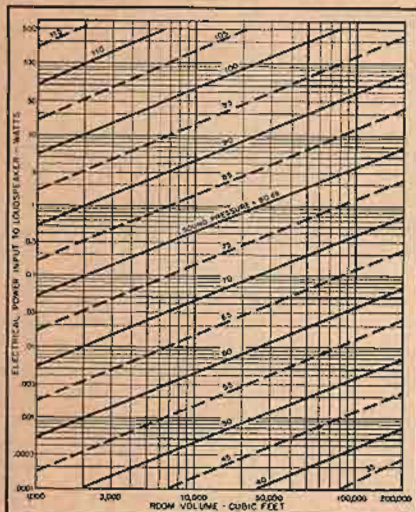
Fig. 14. Loudspeaker power input required for various sound levels, based on 3 per cent efficiency.
