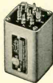
HIGH-FIDELITY INPUT TRANSFORMER, WF-20 , for low impedance microphone, pickup or line to grid. Primary impedance 50, 125/150, 200, 250, 333, 500/600 ohms. Secondary impedance 50,000 ohms. Frequency response 30-20,000 cps. ± 2 db. Negligible harmonic and intermodulation distortion. Grey enamel cast case with phenolic terminal board and tapped holes for flush mounting. 2" high by 1¼" square.
