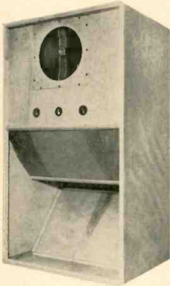
Fig. 4. Complete assembly of speaker unit in back-loading cabinet for use as manual reproducer.
