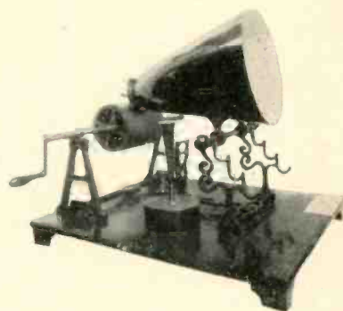
Fig. 7-3. The phonautograph of Leon Scott de Martinville. (Courtesy The Smithsonian Institution).
