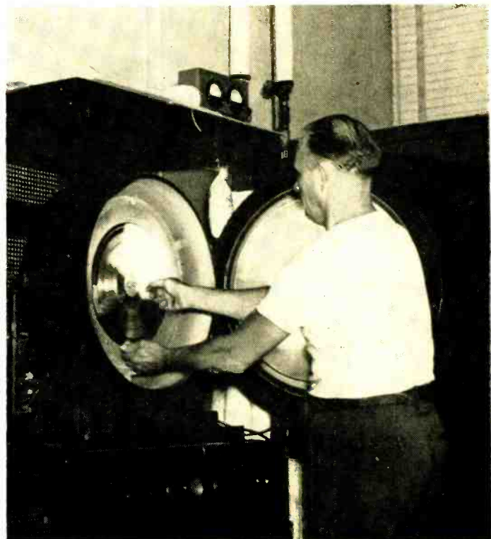
Fig. 2. Operator removes the gold-sputtered master from one of the three vacuum sputtering units.
