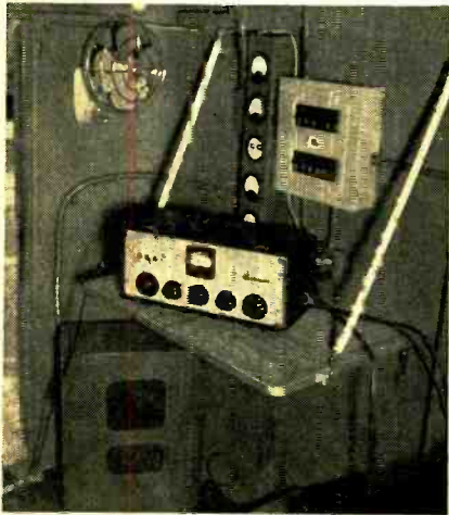
The microphone and audio mixer is a Magnecord PT6-P. It can be operated inside or outside the truck. Below the Magnecord mixer can be seen a small Jensen bass-reflex baffle equipped with long extension lines so that it can be placed near the subject being photographed.
