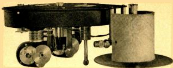
Fig. 14. Selsyn-driven mobile carriage with transducer mounted. This unit simulates aircraft or ship.
