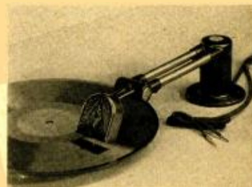
Fig. 2. Early commercial magnetic pickup, showing similarity in construction to acoustic model.
