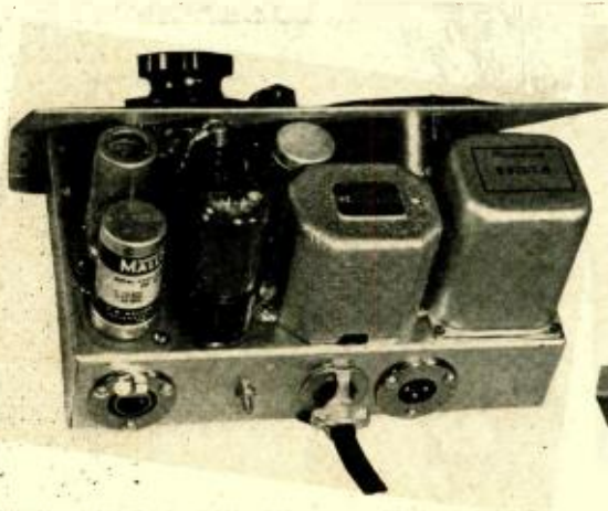
Fig. 8 (left). Top view of amplifier chassis, to show placement of major components. Fig. 9 (right). Under-chassis view of the amplifier.
