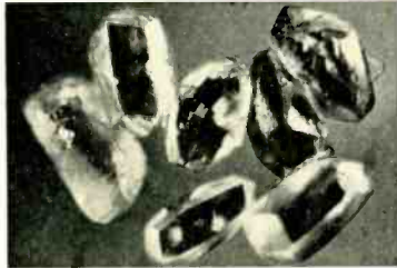
Fig. 1. Small fine industrials. Selected whole diamonds used in manufacture of playback styli. Preferred to cleavages due to greater structural strength. Weight before processing 0.2 gm; after processing, 0.04 gm.
