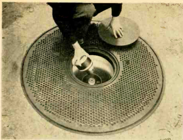
Fig. 1. Ground loudspeaker with protective cover in place, and showing access plate which permits easy removal of driver unit for maintenance.
