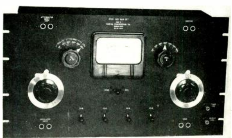
Fig. 6. Cinema 1901 Transmission Measuring Set.
