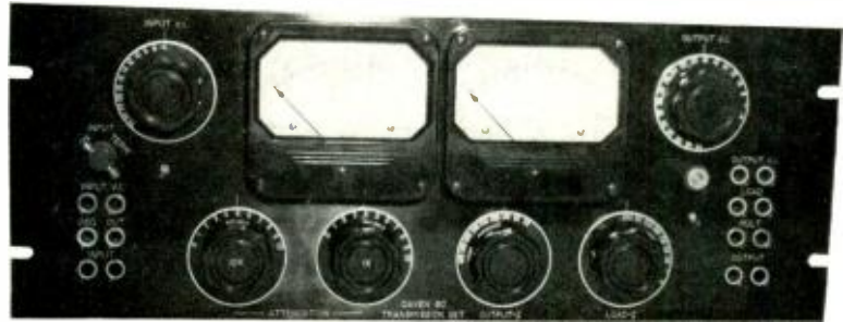
Fig. 5. Daven 6C Transmission Measuring Set.
