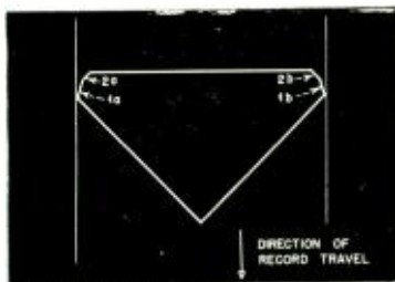
Fig. 8. Cross-section of an Anti-Noise Modulation Stylus having the leading facet 1a and 1b 0.0002" in width; and trailing facet 2a and 2b 0.0001" wide.
