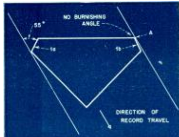
Fig. 3a. Same stylus cross-section in groove whose slope is 30°. Burnishing facet 1a forms angle of 55° with adjacent wall. Facet 1b cannot burnish with groove slope in excess of its basic angle. In fact, the edge formed by the meeting of cutting face and burnishing facet (A) will tear the adjacent groove wall.
