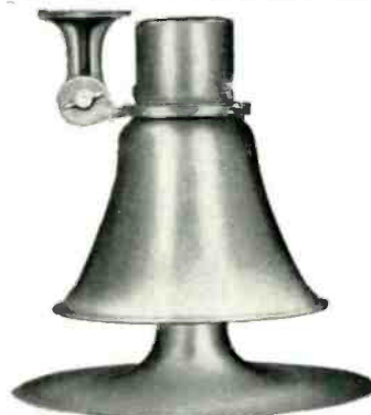
NEW RADIAL RE-ENTRANT SPEAKER , excellent for all types of industrial sound installations. Provides superlative and complete speech intelligibility by efficiently over-riding factory high noise levels. Frequency response 300-6000 cps. Handling capacity 25 watts continuous, 35 w. peak. Has mounting bracket. Size 12" wide by 12½" high.
