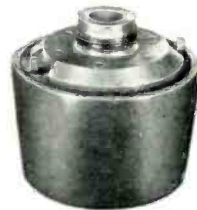
NEW SPÉCIAL PM HORN UNIT having Alnico V magnet ring, completely watertight, housed in a heavy aluminum spinning. Provides extremely high efficiency reproduction with minimum input. Handling capacity 35 watts continuous, 60 w. peak.
