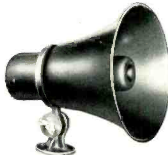
NEW SMALL RE-ENTRANT HORNS , extremely efficient for factory inter-com and paging systems; for sound trucks, R.R. yards and all other industrial installations where high noise levels are prevalent. Watertight, corrosion-proof, easily installed. Two new models — type RE-1½, complete with Baby Unit, handles 25 watts, covers 300-6000 cps; type RE-12, complete with Dwarf Unit, handles 10 watts, freq. response of 400-8000 cps.
